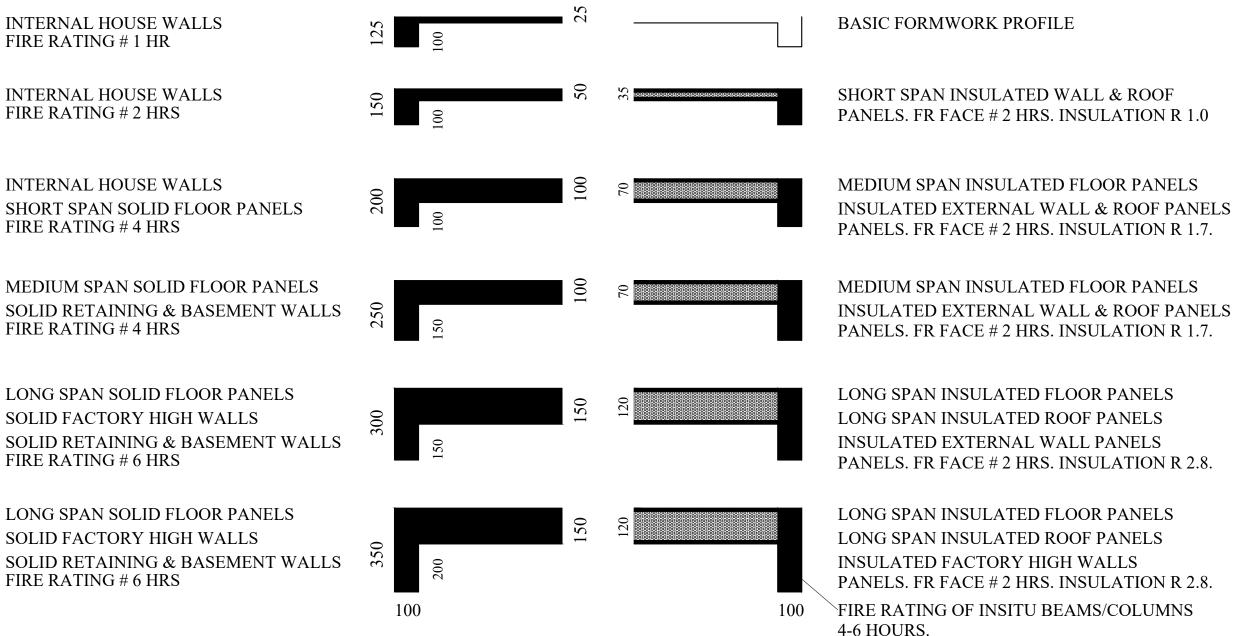
ALL CONCRETE REINFORCED WITH STEEL FIBRES (MADE FROM RECYCLED STEEL). 40- 60 MPA. INSULATION FROM RECYCLED PLASTIC. ACOUSTIC INSULATION CAN BE SUBSTITUTED FOR SOUND RATINGS.
